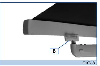
$2^{\circ}$  Using the level (B), positioned near the tip of the arm, check that the terminal is perfectly horizontal. If not, adjust the rod with the plastic ring in the support that corresponds to the arm that is not level, following the procedure described previously.
