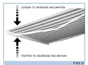
1-Adjust the awning inclination suing the rod with the plastic ring (Fig. 1 - A -) in both arm supports.
