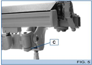
4<sup>o</sup>If not, tighten the grub screw (C) to raise the elbow of the arm, and unscrew it to lower.
